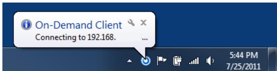
If the connection fails at start-up, or if there is a disruption in the server that causes a disconnection, the application will continue to try to reconnect every 30 seconds. After ten failed reconnect attempts, the Client will enter a standby mode, and the user will need to select “**Reconnect...**” from the menu to try again.
