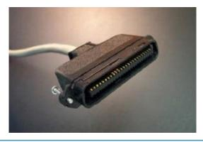
A 180-degree connector is critical to allow the cable to be properly secured to the backplane of the server. The cards in this integration only use the first 24 pairs on the cable. The 25<sup>th</sup> pair is not used.
