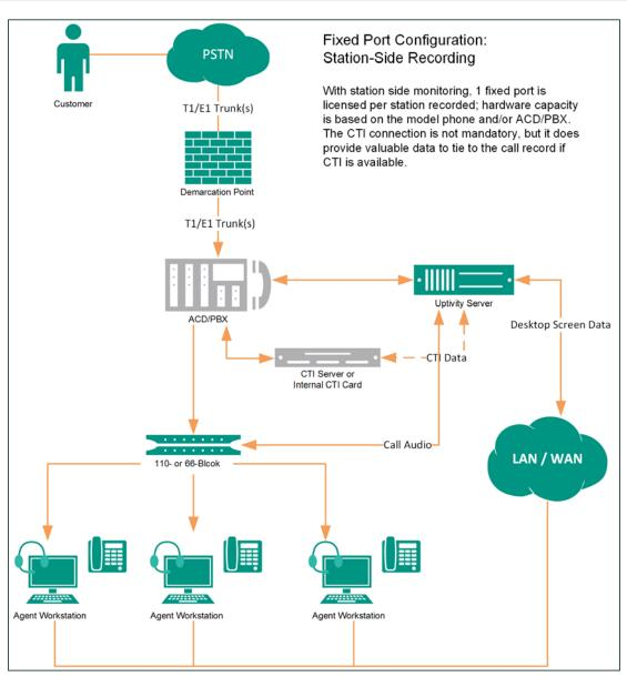
In station-side recording, NICE Uptivity acquires audio from the agent station side of the conversation. Physical audio capture cards installed in the NICE Uptivity recording server have a wired connection to each recorded phone. A CTI connection using TSAPI can provide tighter call control and additional metadata for each call.
