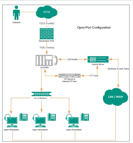
In Open Port/Service Observe recording, NICE Uptivity uses the Avaya Service Observe or Single Step Conference feature to record. Audio capture cards in the recording server are connected to the Avaya PBX through a T1/E1 tie line or through direct analog lines. With appropriate ACD/PBX permissions, these ports can record any device in the system. Since these channels have dial tone at the PBX level, they can also be used to play audio back to specified devices.
