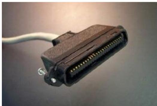
A 180-degree connector is critical to allow the cable to be properly secured to the backplane of the server. The cards in this integration only use the first 24 pairs on the cable. The 25<sup>th</sup> pair is not used.
