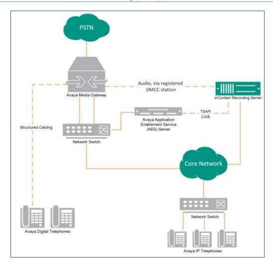
A DMCC recording scenario uses media redirection from Avaya to record calls without the use of physical connections to the inContact WFO recording server other than standard network connections. inContact WFO supports DMCC using service observe (SO), single step conference (SSC), and multiple registration (MR). TSAPI is used in all DMCC recording integrations for call control, messaging, and metadata.
