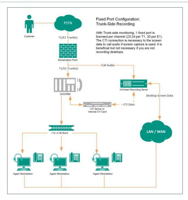
In a trunk-side recording scenario, physical audio capture cards installed in the inContact WFO recording server have a wired connection to each T1/E1 trunk to be recorded, and record from the trunk side of the conversation. A CTI connection using TSAPI can provide events on which to base recording decisions as well as additional metadata for each call.
