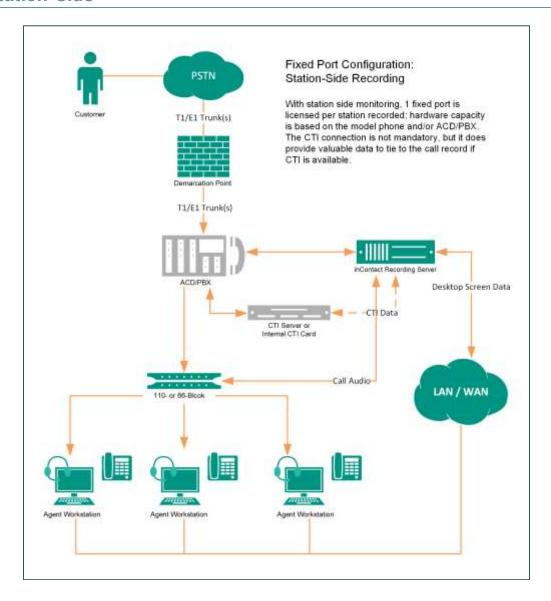
In a station-side recording scenario, inContact WFO acquires audio from the agent-station side of the conversation. Physical audio capture cards installed in the inContact WFO recording server have a wired connection to each recorded phone. A CTI connection using TSAPI can provide tighter call control and additional metadata for each call.
