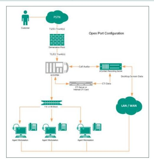
In an Open Port/Service Observe recording scenario, inContact WFO uses the Avaya Service Observe or Single Step Conference feature to record. Audio capture cards in the recording server are connected to the Avaya PBX through a T1/E1 tie line or through direct analog lines. With appropriate ACD/PBX permissions, these ports can record any device in the system. Since these channels have dial tone at the PBX level, they can also be used to play audio back to specified devices.
